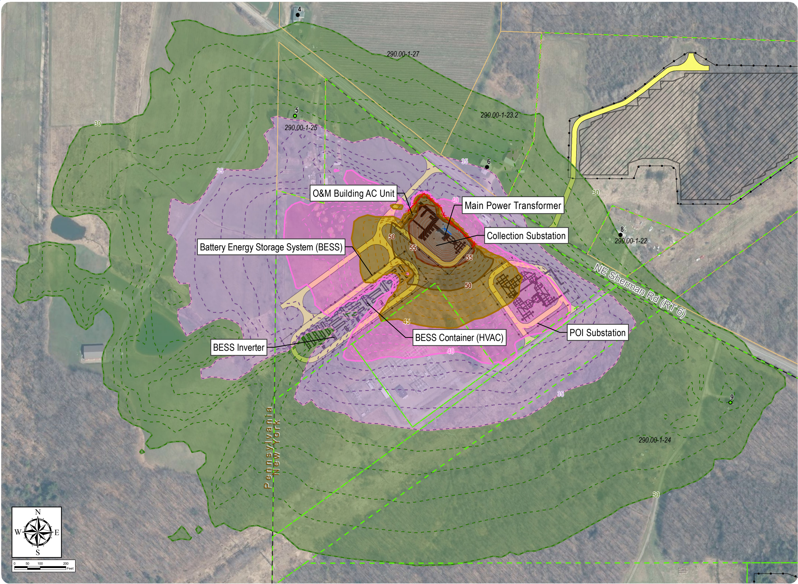
Figure S7-2: Sound Contours - Collection Substation
