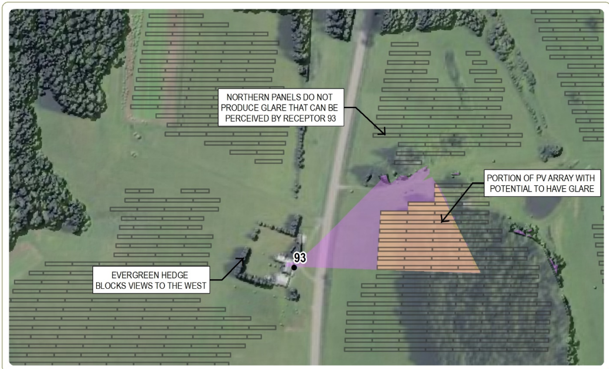
Inset Figure 4. Final model input data for Receptor 93 (shown in orange). These model input data were developed based on the results of the observation point viewshed analysis (shown in purple, for reference), the results of the field verification, and the results of the Preliminary Glare Analysis. Proposed photovoltaic (PV) panels are outlined in dark gray.
